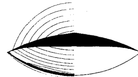
Fig. 15 Mach 4 waverider; pressure isolines and exact shock location.
